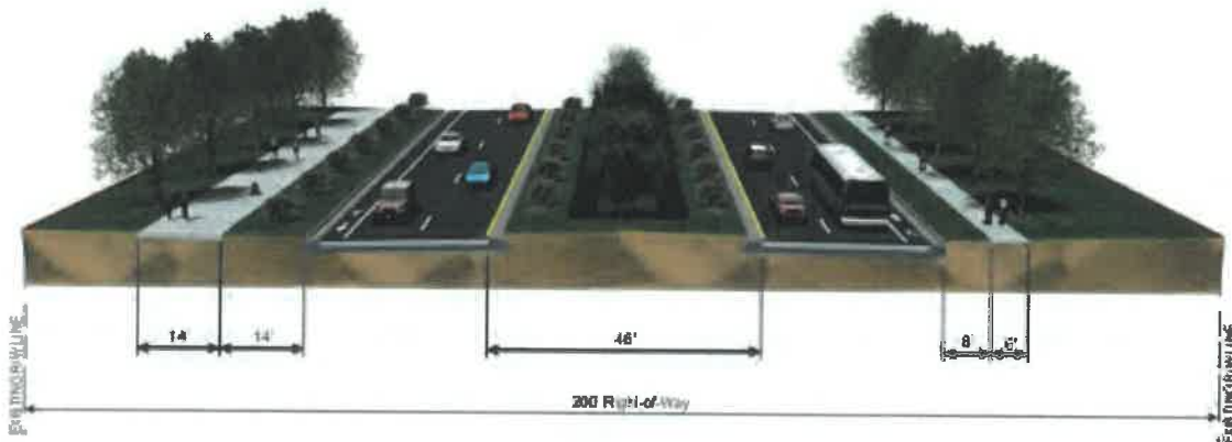
Figure 2. Typical Roadway Section - 200' Right-of-Way
