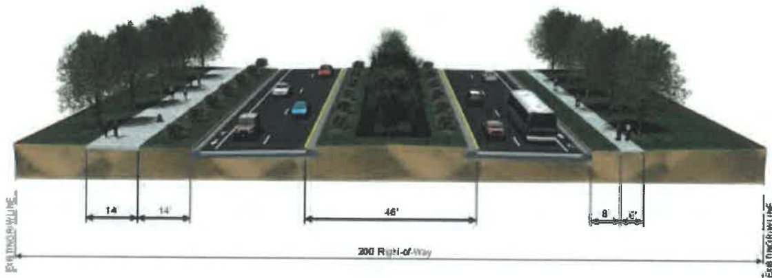
Figure 2. Typical Roadway Section - 200' Right-of-Way
