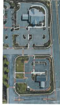
Pedestrian connections between parking rows and buildings
